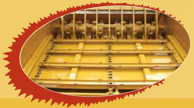
**Access Door/Screens:** The large access door allows easy accessibility to the flail tube, screens and transition auger. Switching from fan discharge to conveyor discharge is also accomplished here, and only takes a few minutes to do the conversion. Screens are available in 2", 3" and 4" round as well as 4 1/2" x 9" and 6 1/2" x 9"
